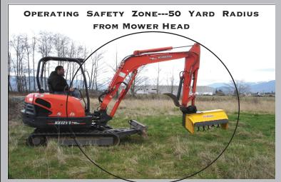
STOP! AND ALLOW ALL VEHICLES TO PASS THROUGH OPERATING "SAFETY ZONE" BEFORE CONTINUING CUTTING. OPERATOR AWARENESS IS KEY TO SAFE OPERATION. NEVER OPERATE OR CON-TINUE TO OPERATE THIS MACHINE WHEN THERE IS A PERSON OR VEHICLE WITH-IN A 50 YARD RADIUS OF THE CUTTING OPERATION. IF A PERSON COMES IN-SIDE YOUR OPERATING "SAFETY ZONE" (50 YARD RADIUS) SHUT THE MACHINE DOWN.
